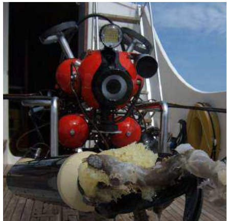
Figure 4. Freshly collected samples in the grabber of the Multip Pluto ROV
